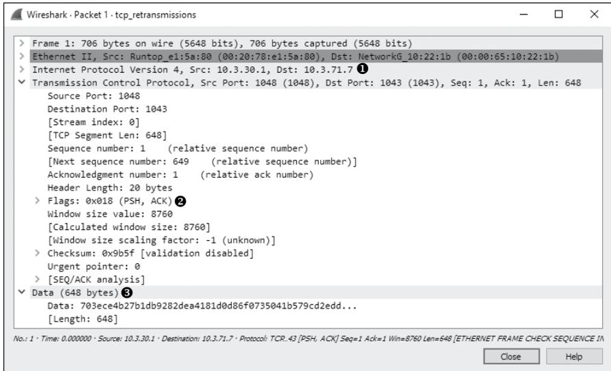
Figure 11-2: A simple TCP packet containing data
