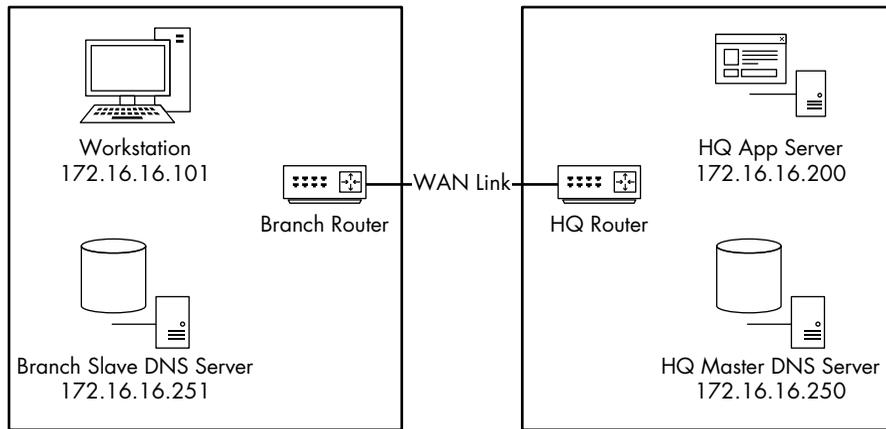
Figure 10-29: The relevant components for the stranded branch office issue
