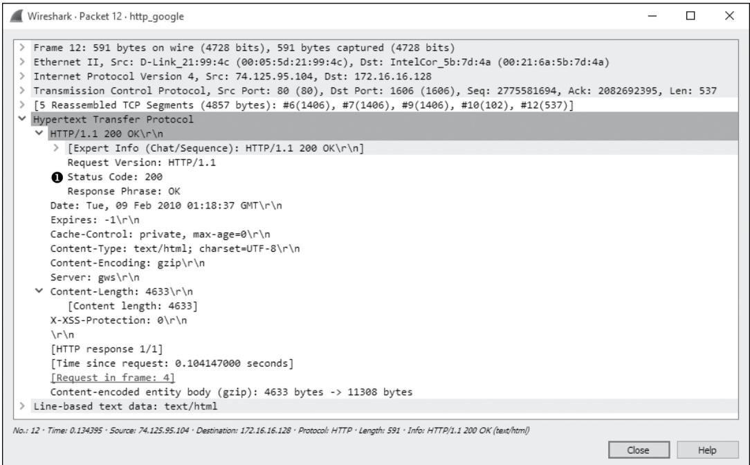
Figure 9-24: Final HTTP packet with response code 200
