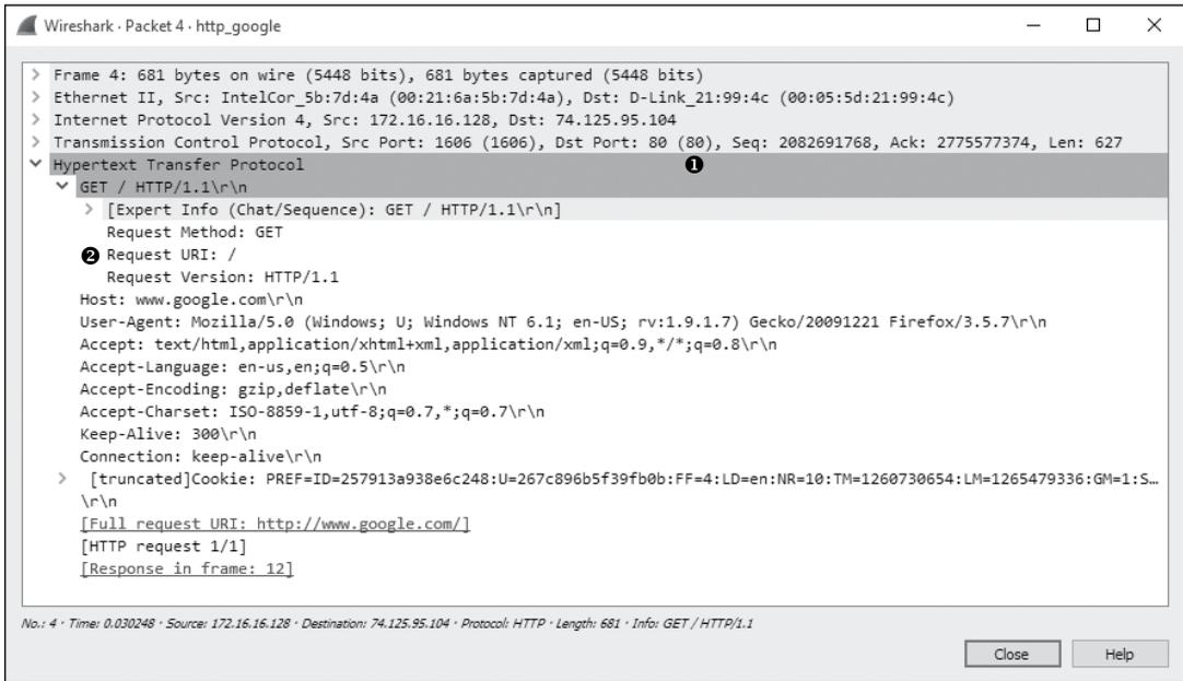
Figure 9-22: The initial HTTP GET request packet
