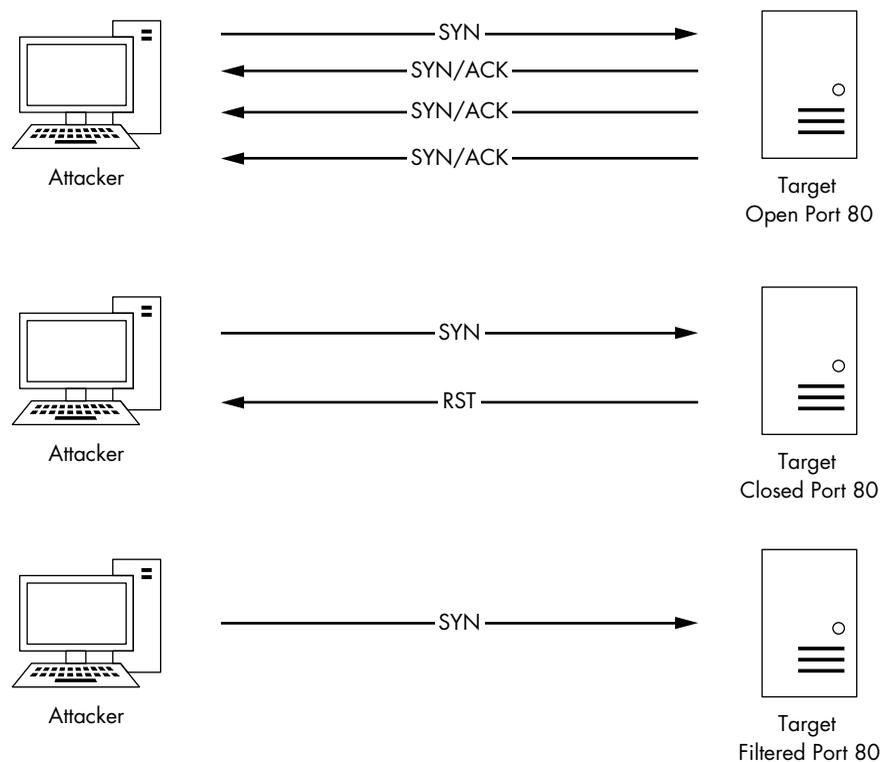
Figure 12-1: Possible results of a TCP SYN scan
