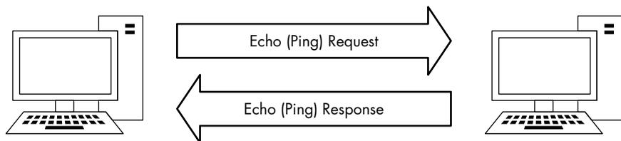
Figure 7-29: The ping command involves only two steps.
