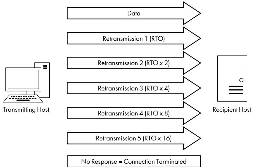
Figure 11-1: Conceptual view of the TCP retransmission process
