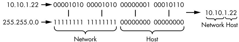
Figure 7-8: The netmask determines the allocation of the bits in an IP address.
