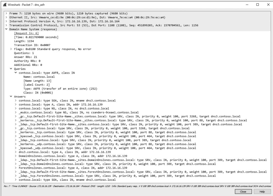
Figure 9-21: The DNS full zone transfer occurring
