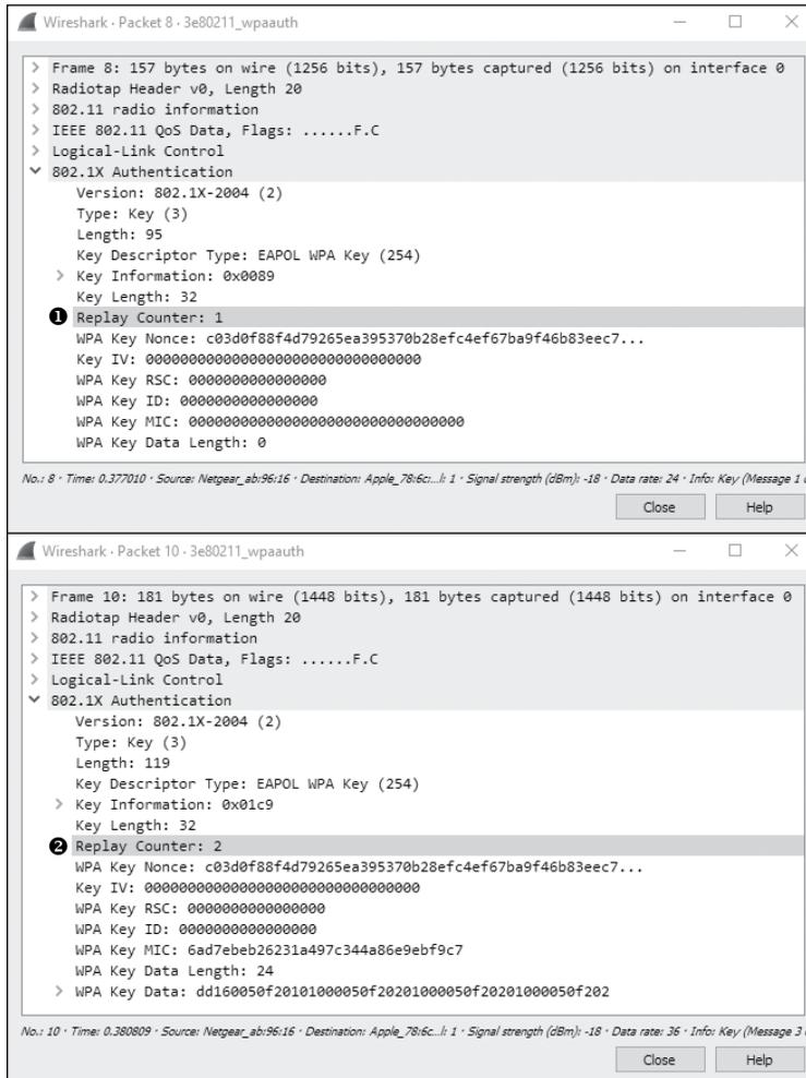
Figure 13-18: The Replay Counter field helps us pair challenges and responses.
