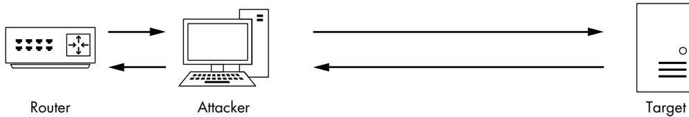
Figure 12-10: ARP cache poisoning as an MITM attack
