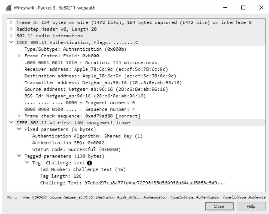
Figure 13-11: The WAP issues challenge text to the wireless client.
