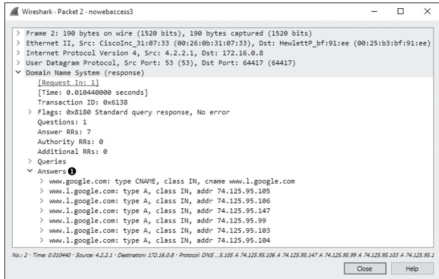
Figure 10-22: DNS reply with multiple A records
