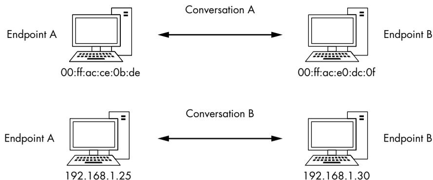
Figure 5-1: Endpoints and conversations on a network
