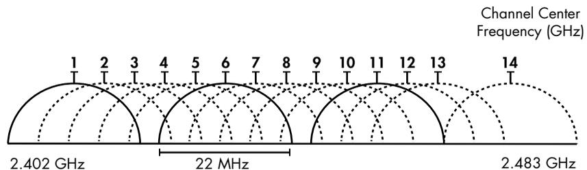
Figure 13-2: There is overlap between channels due to limited spectrum space.
