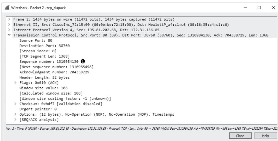
Figure 11-9: The sequence number of this packet is not what was expected.
