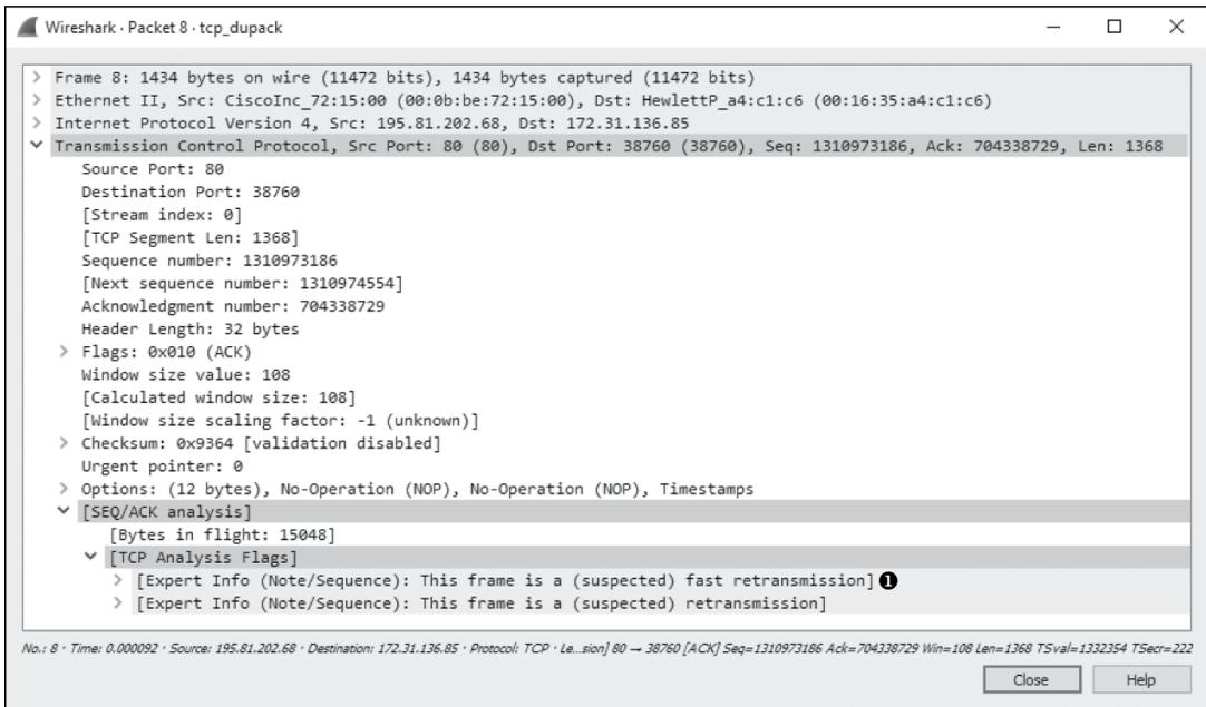
Figure 11-12: Three duplicate ACKs cause this fast retransmission of the lost packet.
