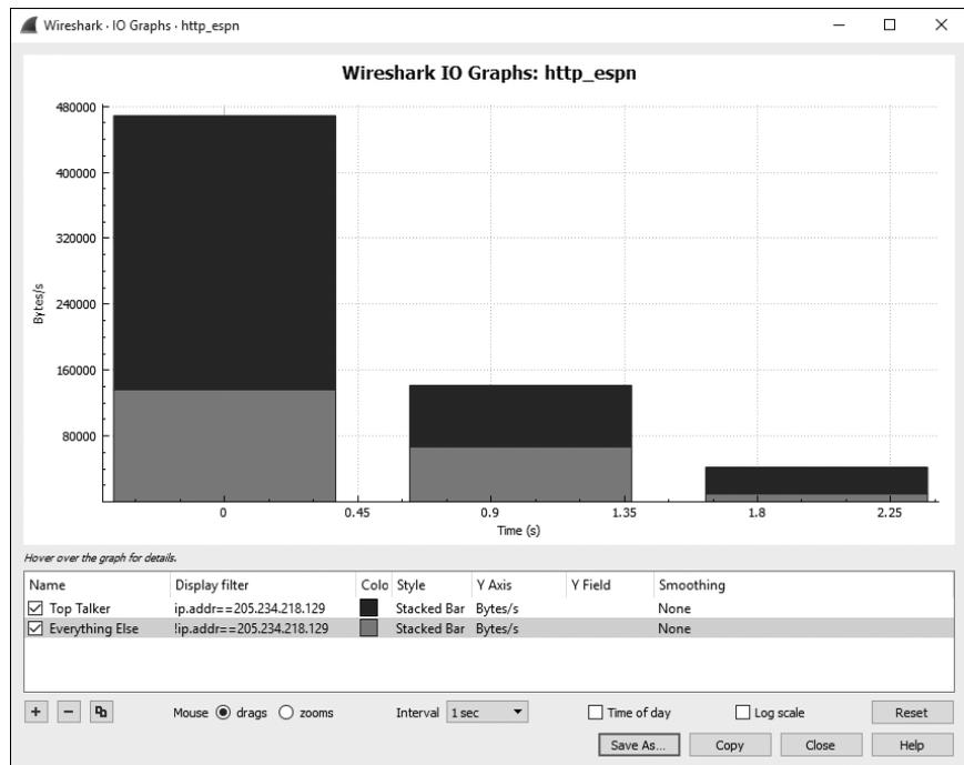
Figure 5-20: An IO graph showing IO of two separate devices.
