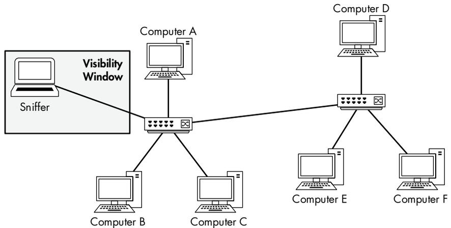
Figure 2-4: The visibility window on a switched network is limited to the port you are plugged into.
