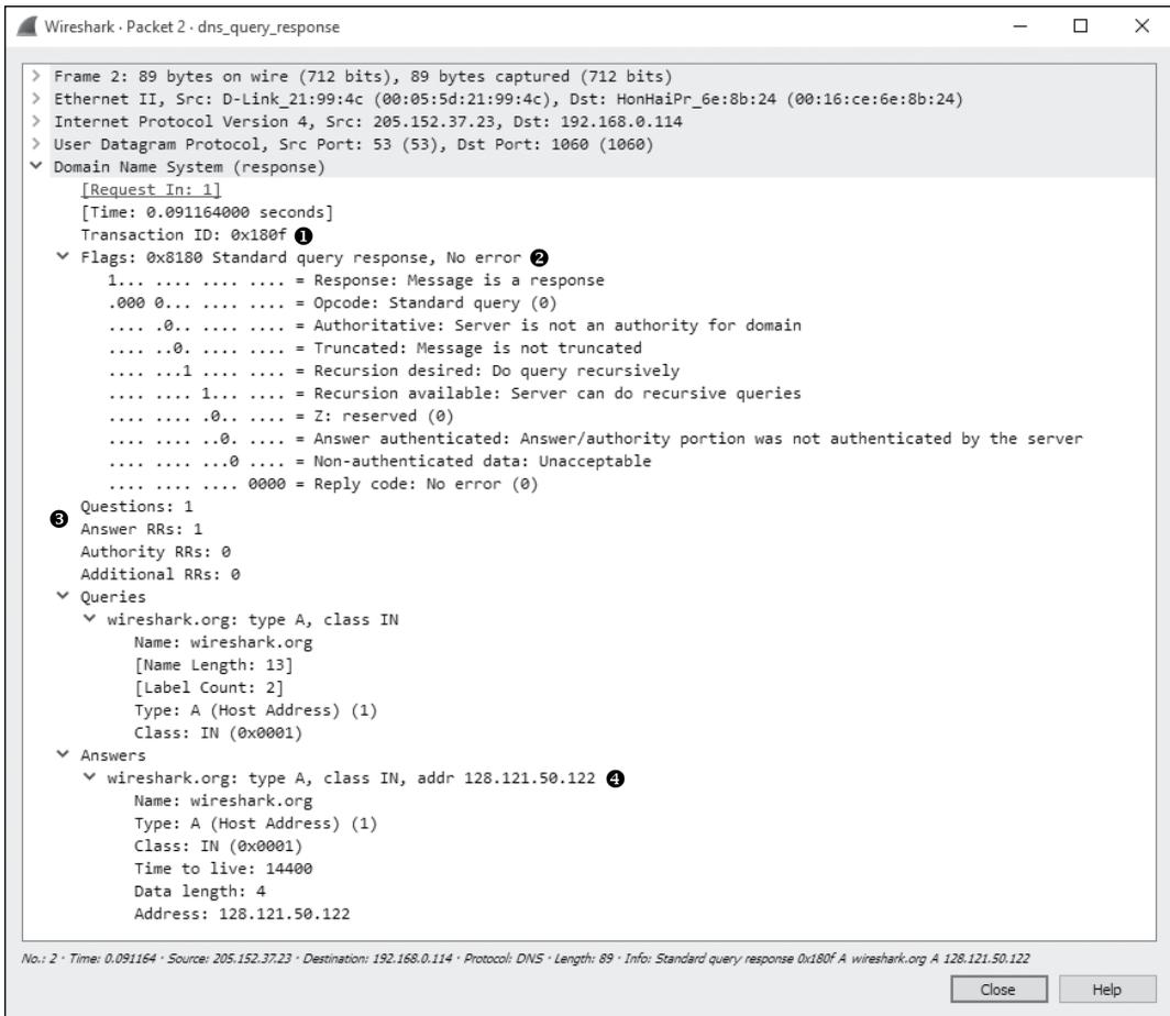
Figure 9-12: The DNS response packet
