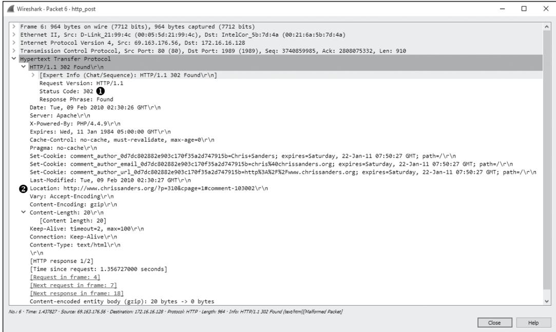
Figure 9-26: HTTP response 302 is used to redirect.
