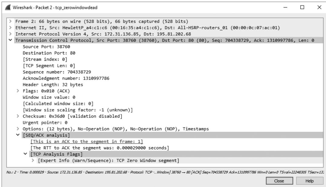
Figure 11-19: A zero window packet halts data transfer.
