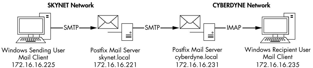
Figure 9-29: Tracking an email from sender to recipient
