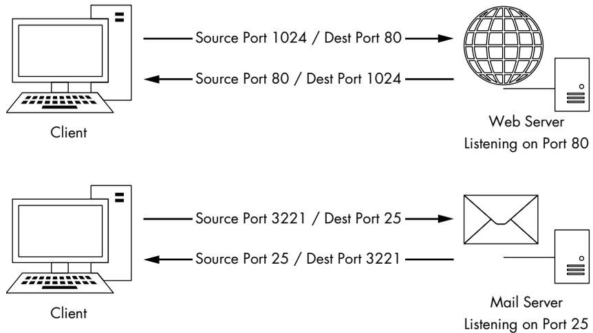
Figure 8-2: TCP uses ports to transmit data.
