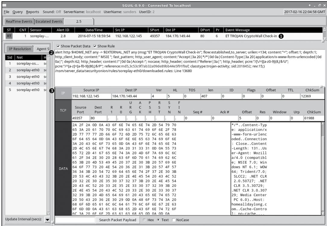
Figure 12-31: This IDS alert indicates a CryptoWall 4 infection.
