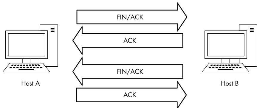
Figure 8-9: The TCP teardown process
