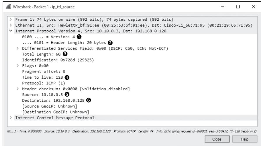
Figure 7-11: The IP header of the source packet
