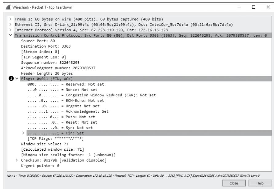
Figure 8-10: The FIN/ACK packet initiates the teardown process.
