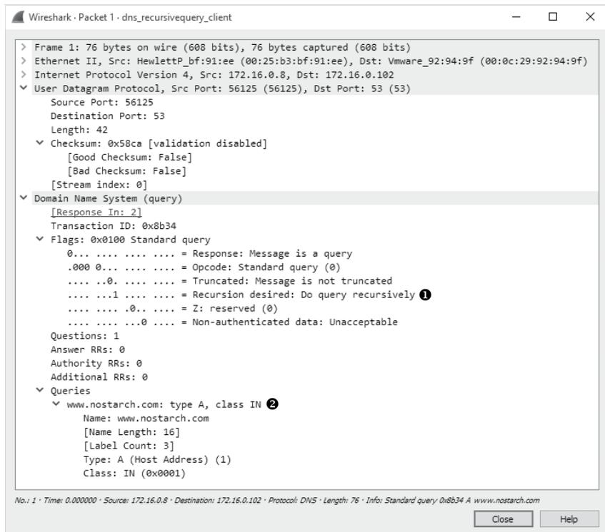
Figure 9-13: The DNS query with the Recursion desired bit set
