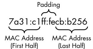
Figure 7-17: The interface ID utilizes an interface MAC address and padding.
